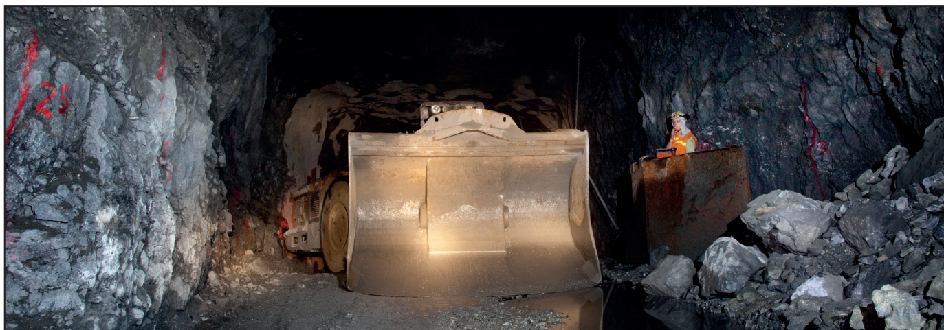
Fig. 3: Load Haul Dump machine in operation on remote control
