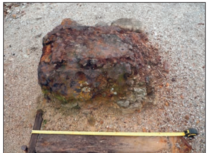
Figure 21. One of four rusted concretions, this one still within its wooden box frame, denoting the base of one of the Cornish stamp batteries, which is a highly rare example of nineteenth century stamp bed formation
