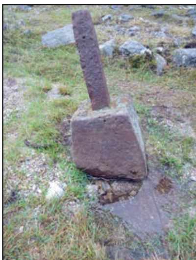
Figure 8. A well-worn short shank stamp shoe found in the vicinity of Lughnure Adit where there was an early dressing floor. See the Perran Foundry Catalogue for similar examples (Trevithick Society 1986, p.13)
