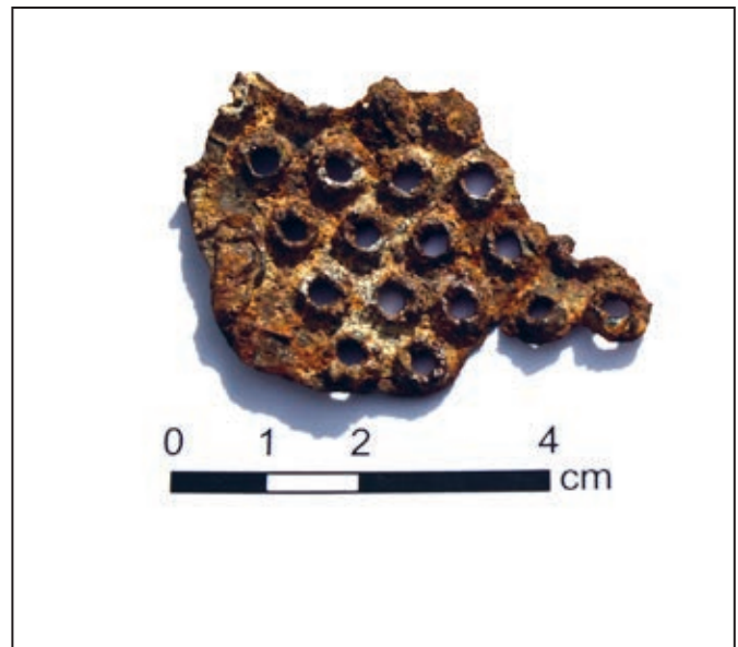
Figure 30. A fragment of stamp screen manufactured from punched iron sheeting, with holes approximately 3 mm (one eighth of an inch) in diameter
