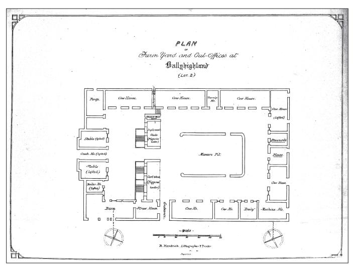
Fig. 9: The farm yard at Ballyhighland which was subjected to costeaning by Captain Barrett. Note the house of Howlin's steward, Clement Sinnott (centre right), and the two circular horse whims generating power to the barn (bottom left) and machinery shed (bottom right). Sale notice of the Ballyhighland Demesne, Find My Past
