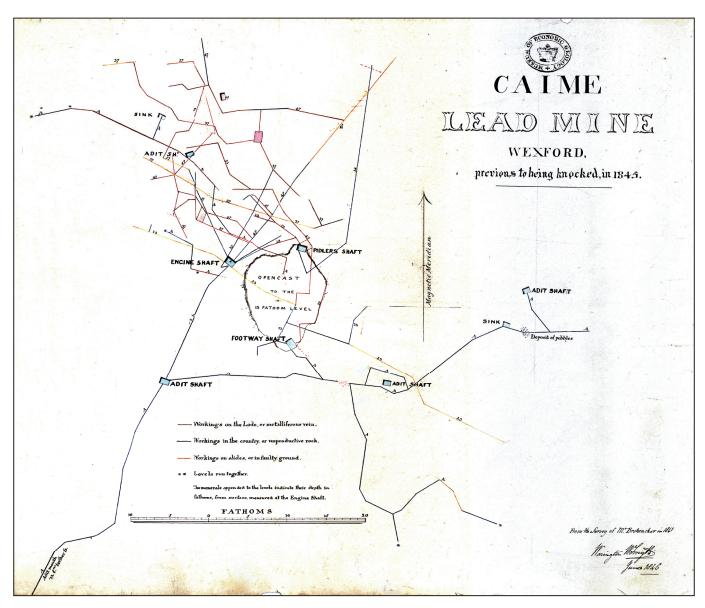
Fig. 10: Plan of Caime Mine dated June 1846, by mining geologist Warington W. Smyth (1817-1890) of the Geological Survey of Great Britain and Ireland, based on a previous survey conducted by Cornishman, Benjamin Brokenshar, in 1841. Courtesy of the Geological Survey of Ireland
