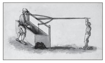
Fig. 5: A hand operated brake jig, such as would have been in use at Caime Mine. Reproduced with kind permission of the Science Museum
