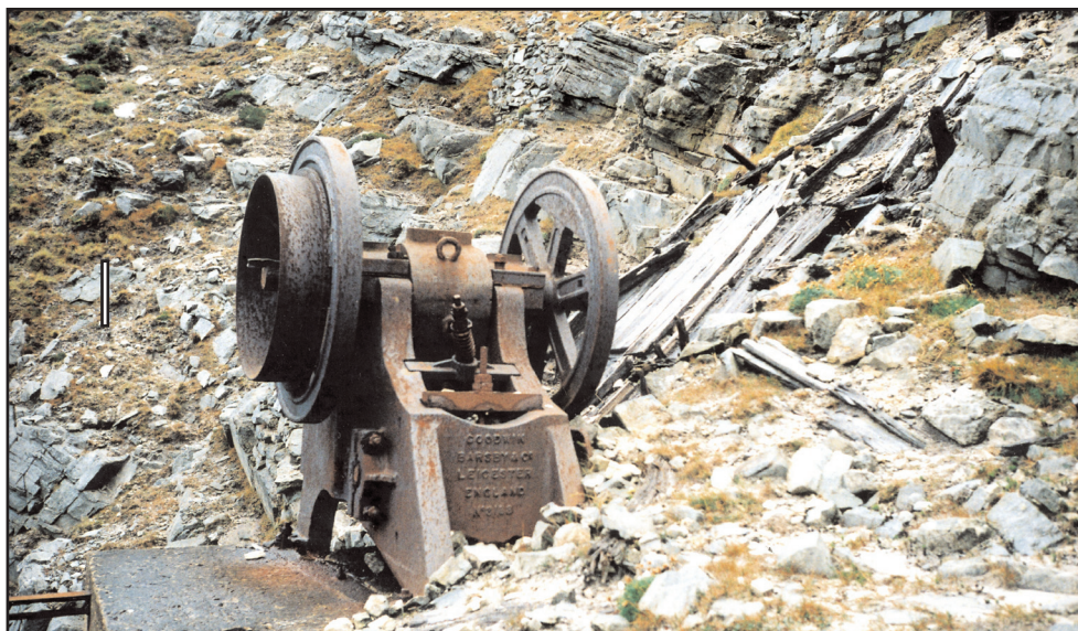
Figure 12. The lower crusher and gearbox and engine, with Rupert Fabby examining the crusher. Photo: Alastair Lings.
