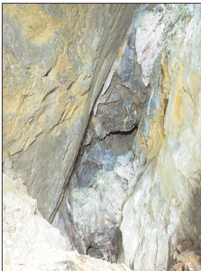
Figure 5. The mineral vein seen on the far side of the open stope. Small openings below and above a large collapsed 'flake' can be seen in the lower half.
