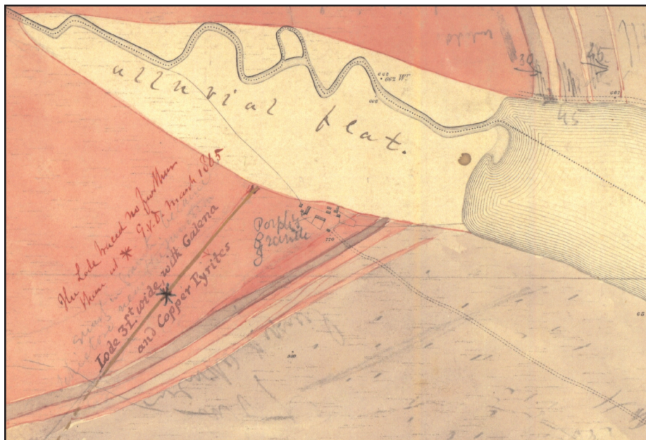
Figure 11. The three main elements of granite and schist are annotated, along with the alluvium filling the valley floor. The line of the vein is illustrated and the spoil heaps are clearly visible beside it. Number 1 is beside the upper level and number 2 beside the lower level (courtesy of Shay Foody).
