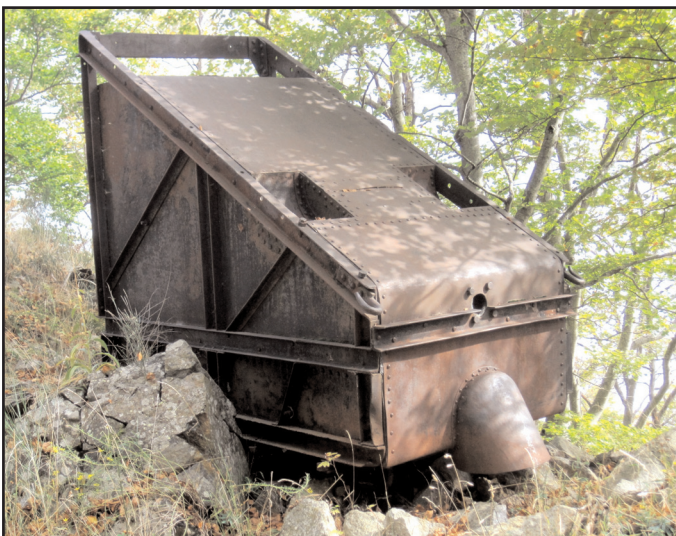
Figure 11 - Water balance tank from the incline at Les Manerots (inverted with undercarriage removed), 2015 (authors' photograph).
