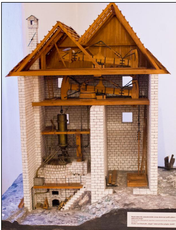
Working model of an atmospheric steam engine built from the plans of Joseph Emanuel Fischer von Erlach at the Slovenské Banské Múzeum, Kammerhof
