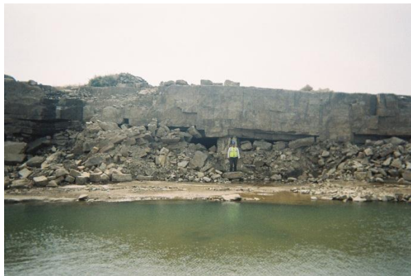
Backfilled workings at Drumkeelan Lower Quarry
