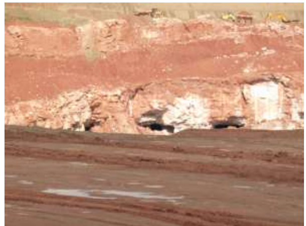
Older underground adits intersected by the opencast pit. (Stephen Callaghan)
