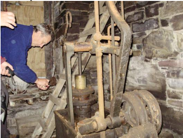
The Cataract for the Steam and Exhaust Valves
