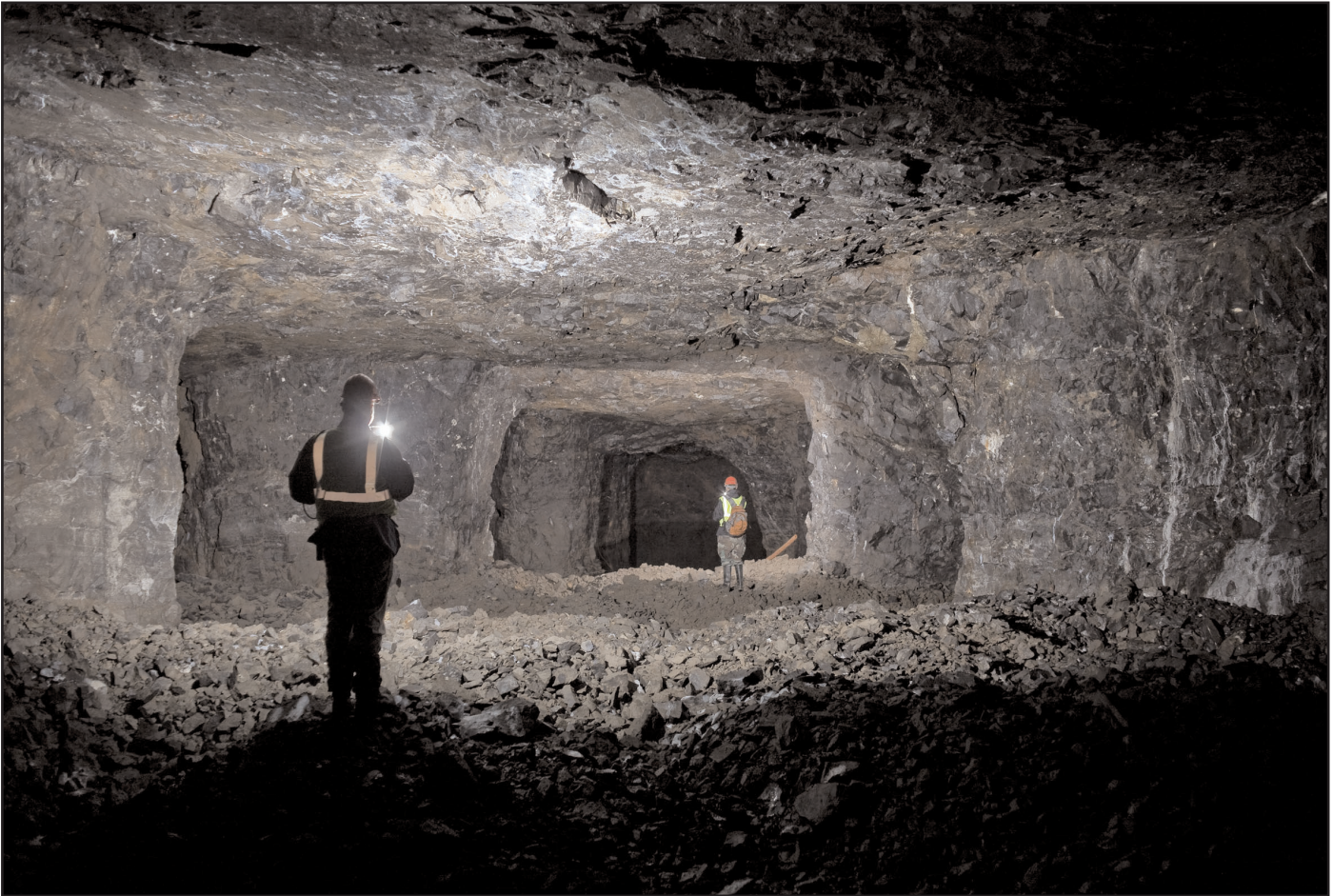
Photo 7 Above. Recent photograph in the western part of the Main Index Bed stall and pillar mining area.
